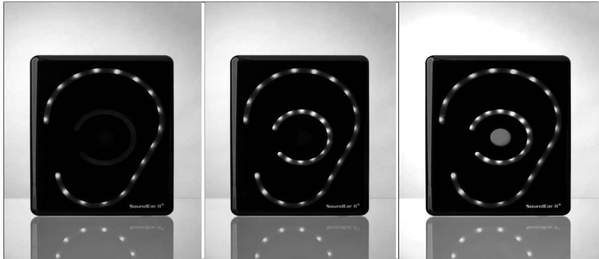
Pic. 2. The device for monitoring the volume of sounds in hospital wards (green – normal, yellow – loud, red – noise).
